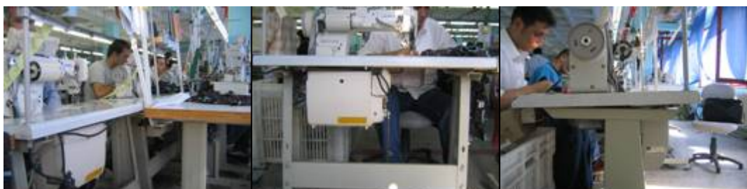
Figure IV.8. Tilting Adjustments in Machine Sewing Workstation
