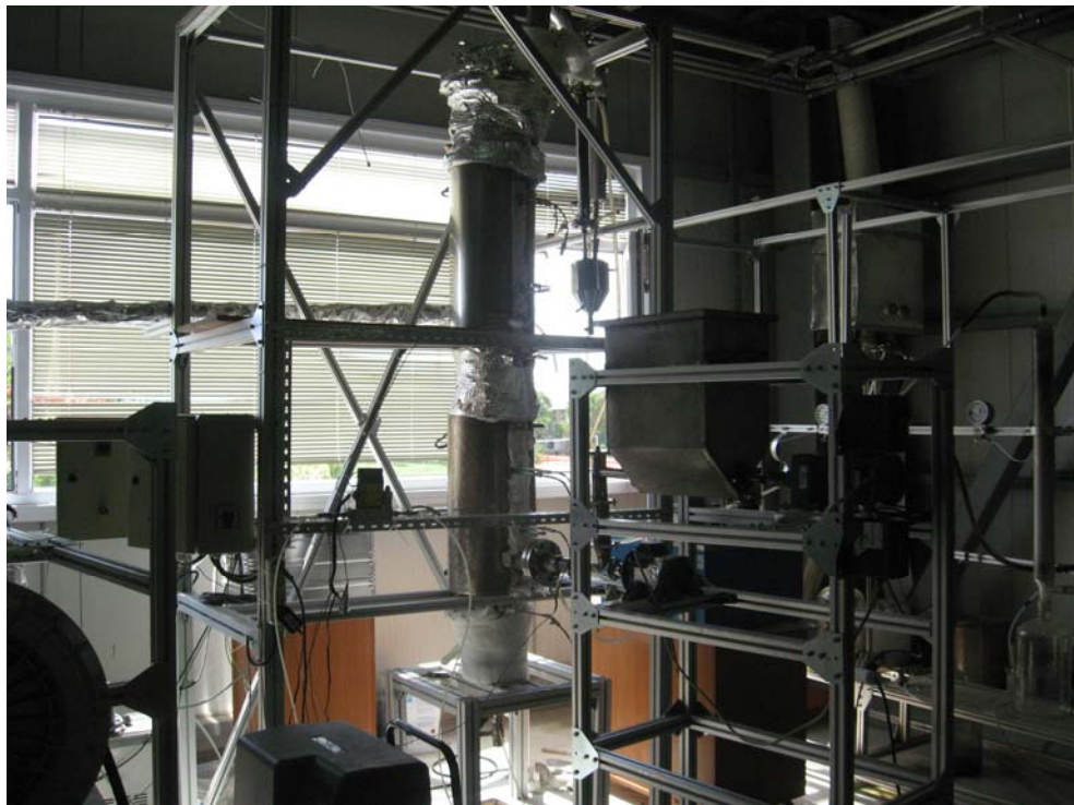
Figure III. 10 Bubbling Fluidized Bed Gasifier System
