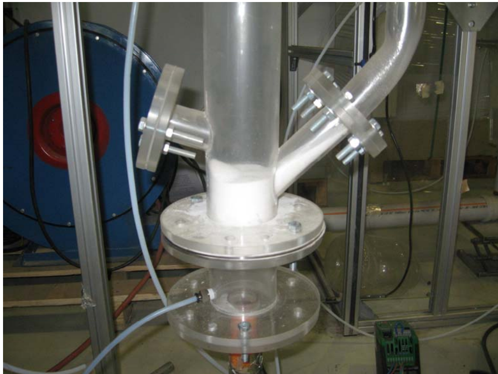
Figure IV.1 The Bed of Cold Fluidized Bed Model
