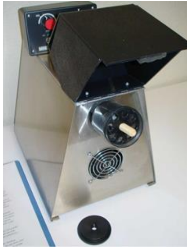
Figure 3.9 Bead beater that is used for ball milling
