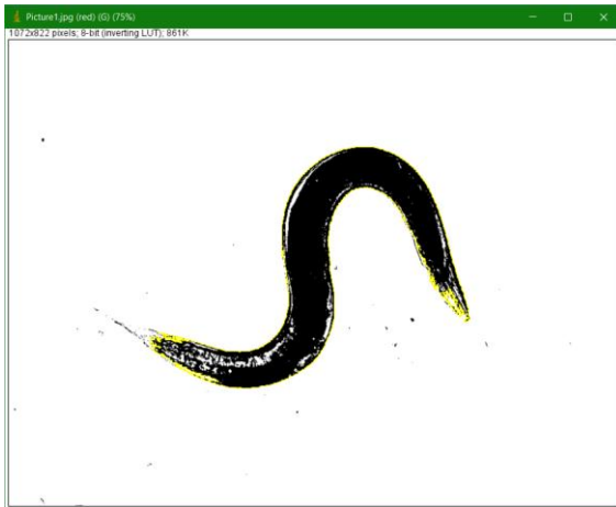
Figure 2.5. Image of nematode after its pixels was inverted and selected with wand tool. Yellow borders designate selected parts of the image.
