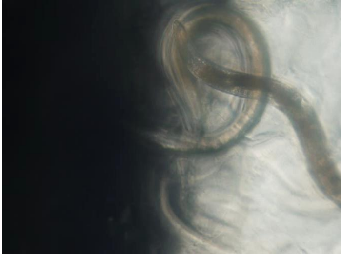
Figure 2.2. Uneven lightning near the borders of a petri dish caused by default stage of IX-71 microscope.
