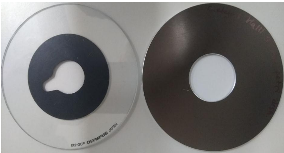
Figure 2.3. On the left, pear shaped stage that casts dark zones on the plates, on the right custom-made stage designed for 35-mm petri dishes.
