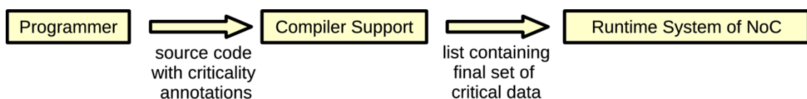
Figure 3.1. The workflow of the compiler-enhanced reliability framework
