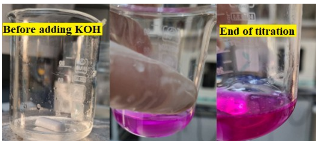
Figure 3.11. Determination of lipase activity by titration of free fatty acids
