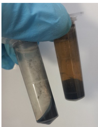
Figure 3.17. Precipitation of proteins by activated carbon
