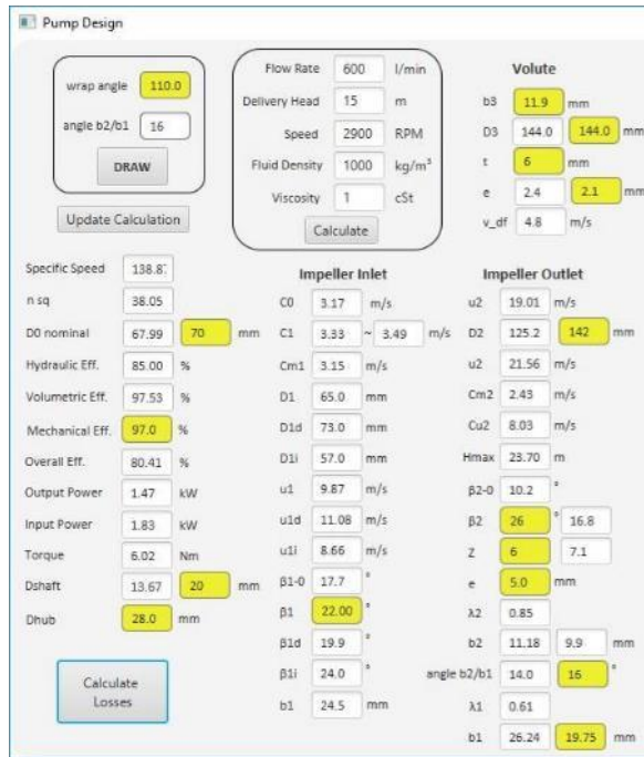
Figure 3.2. Calculation on main dimensions of Pump-1
