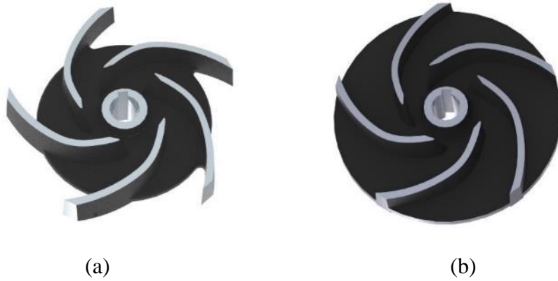
Figure 3.38. Impeller of (a) experimental Pump-3 and (b) predicted and CFD Pump-3
