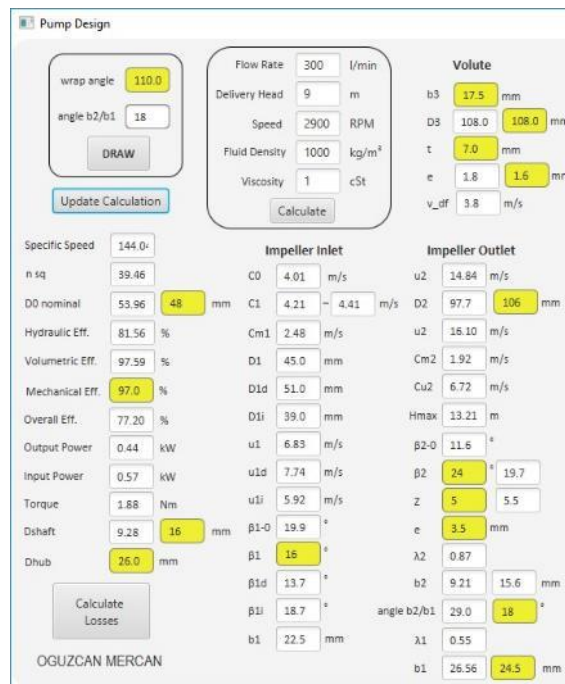
Figure 3.3. Calculation on main dimensions of Pump-2
