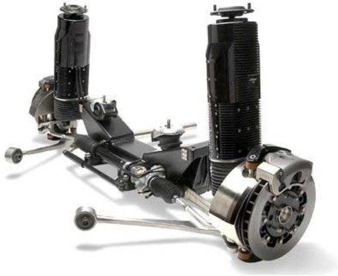
Figure 1.2: Bose active suspension system
