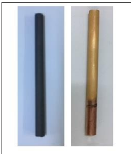
Figure 2.7. Graphite and gold coated copper electrodes (from left to right)
