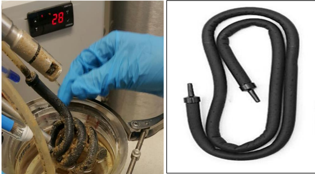
Figure 3.6 Pictures of the flexible diffuser before and after experiments
