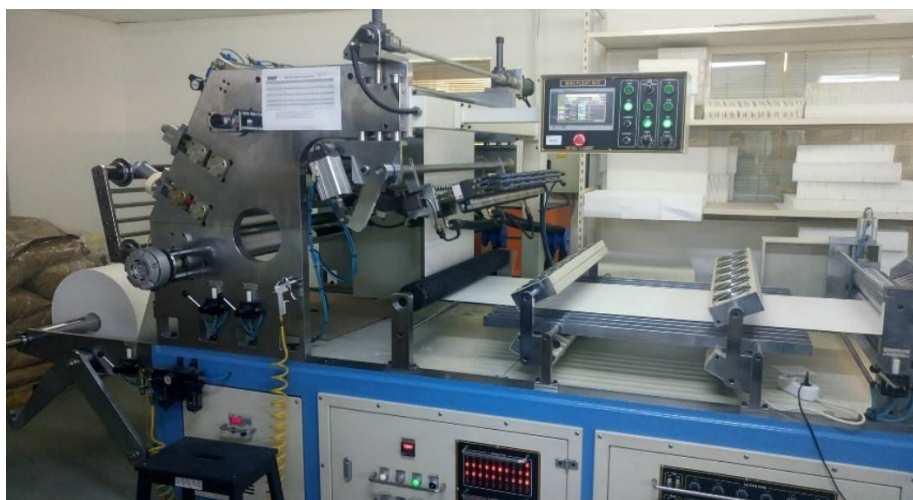
Figure 5.4: Manufacturing System of HEPA Filter Media
